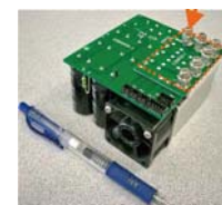
Power conditioner (Power conversion efficiency of 97.5%)
