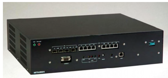
Fig. 1 Prototype for Ethernet OAM/protection functions
